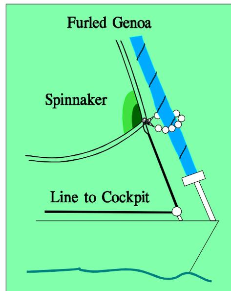
Lead the lazy sheet aft on the other side of the boat, outside the shrouds and lifelines to the turning block, and then forward to a winch.
