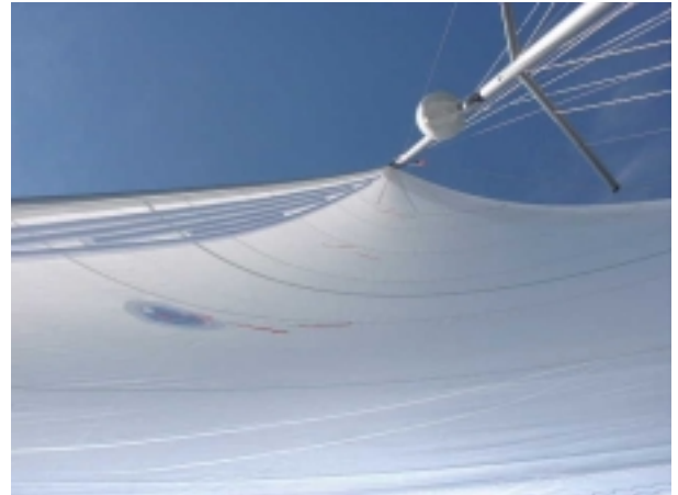
Here the genoa is completely unfurled and trimmed up for sailing upwind in about 8 knots of breeze.
