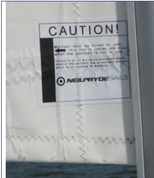
Furling Label on starboard side of mainsail clew patch
