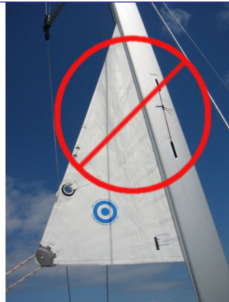
Mainsail with label and sail exposed; INCORRECTLY furled
