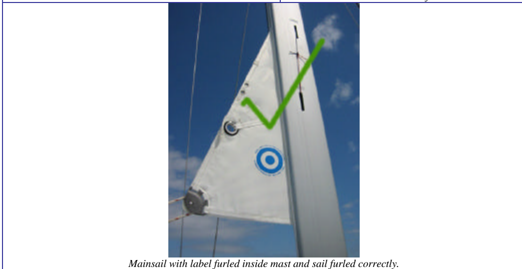
Furling Label on starboard side of mainsail clew patch
