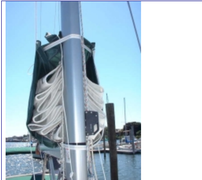
With forward flap folded back inside and secured to the hook and loop strip.
