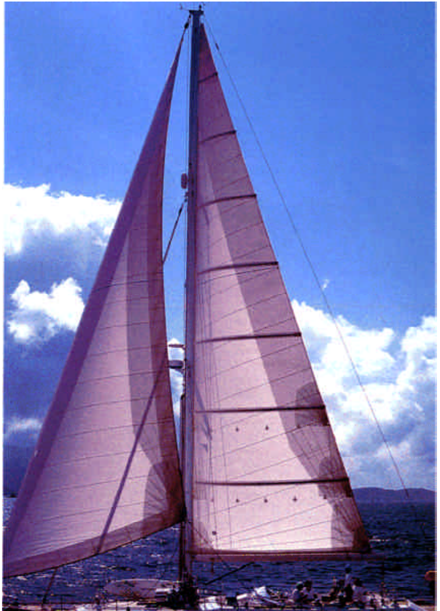
The full length battens create a smooth airfoil that is more easily handled and longer lasting than a traditional main.
