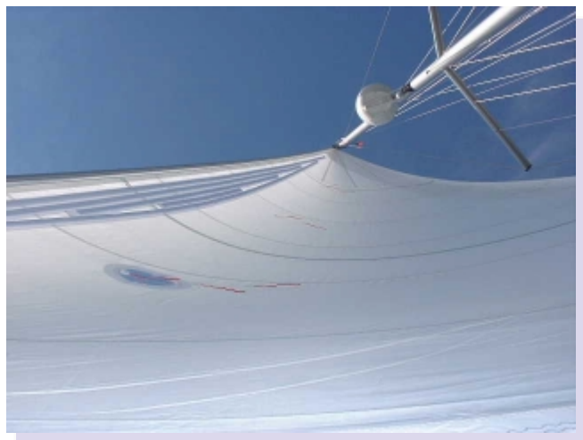
Here the sail is completely unfurled, the amount of shape (camber) is represented numerically and is 16% in the mid-section and 16.7% in the top section.
