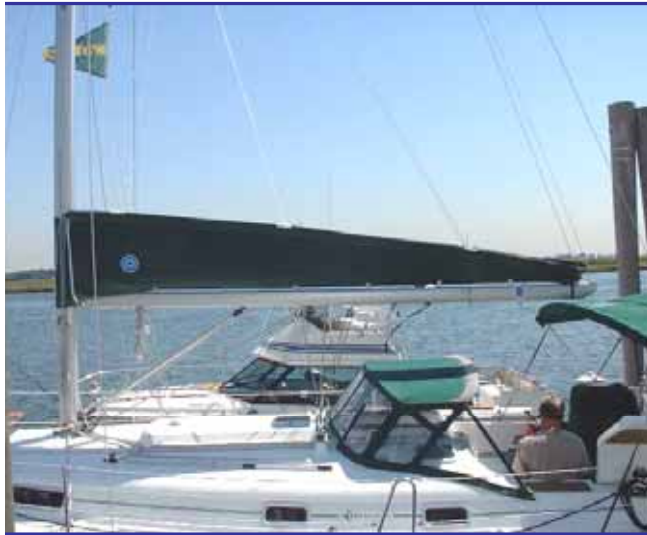
361 Lazy Bag Installed
