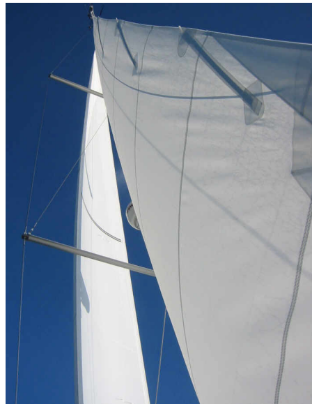
Leech trim, closed hauled and with full size sail. Note location of leech at each spreader
