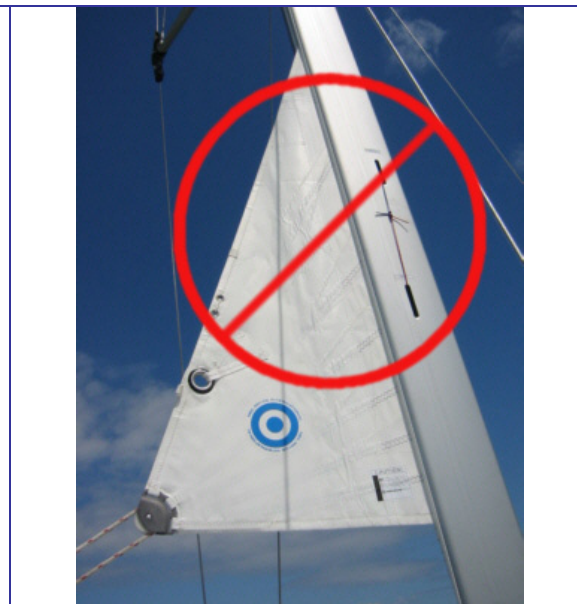
Mainsail with label and sail exposed; INCORRECTLY furled
