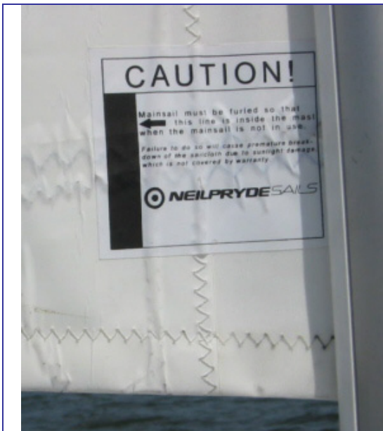
Furling Label on starboard side of mainsail clew patch
