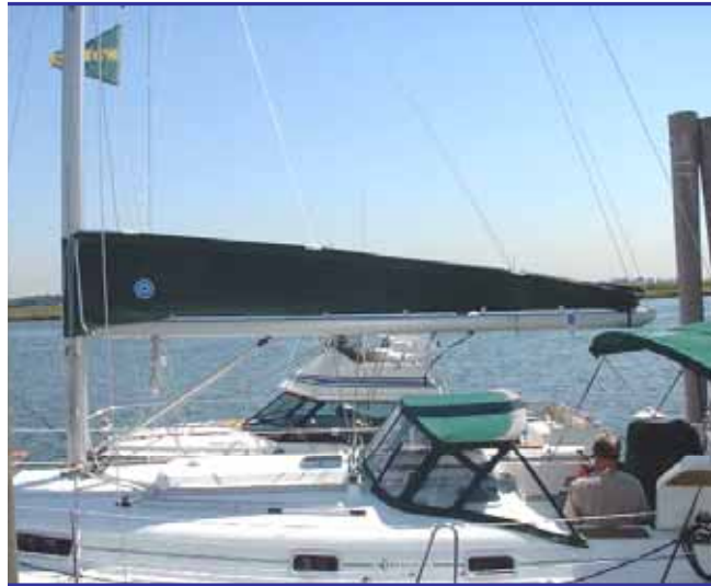
361 Lazy Bag Installed
